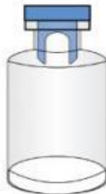
Step 3: When lyophilization is complete the stopper is seated
