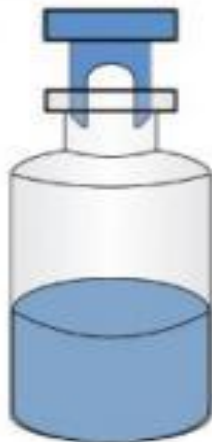
Step 2: Stopper is partially inserted and the vial is placed in a lyophilizer
